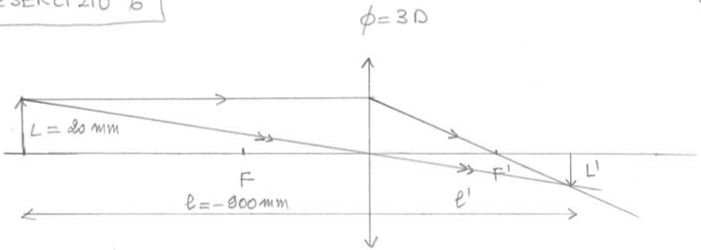
$$\frac{1}{e'} = \frac{1}{e} + \phi = -\frac{1}{900} + \frac{3}{1000} = \frac{-10 + 27}{9000} = \frac{17}{9000} \text{ mm}^{-1} \Rightarrow$$
