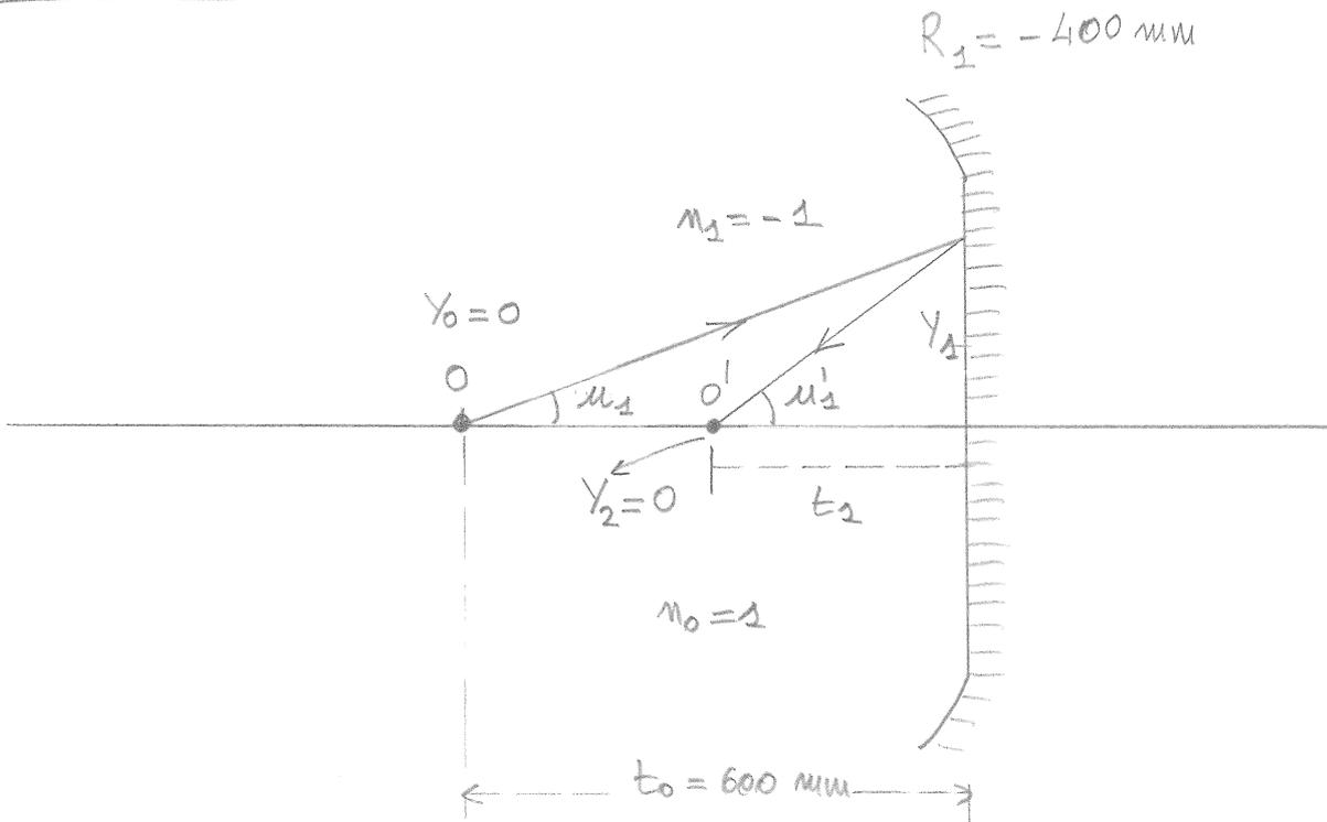
$$\gamma_1 = \gamma_0 + t_0 \mu_1 \Rightarrow \gamma_1 = t_0 \mu_1 \Rightarrow \gamma_1 = 600 \mu_1 \text{ mm}$$
