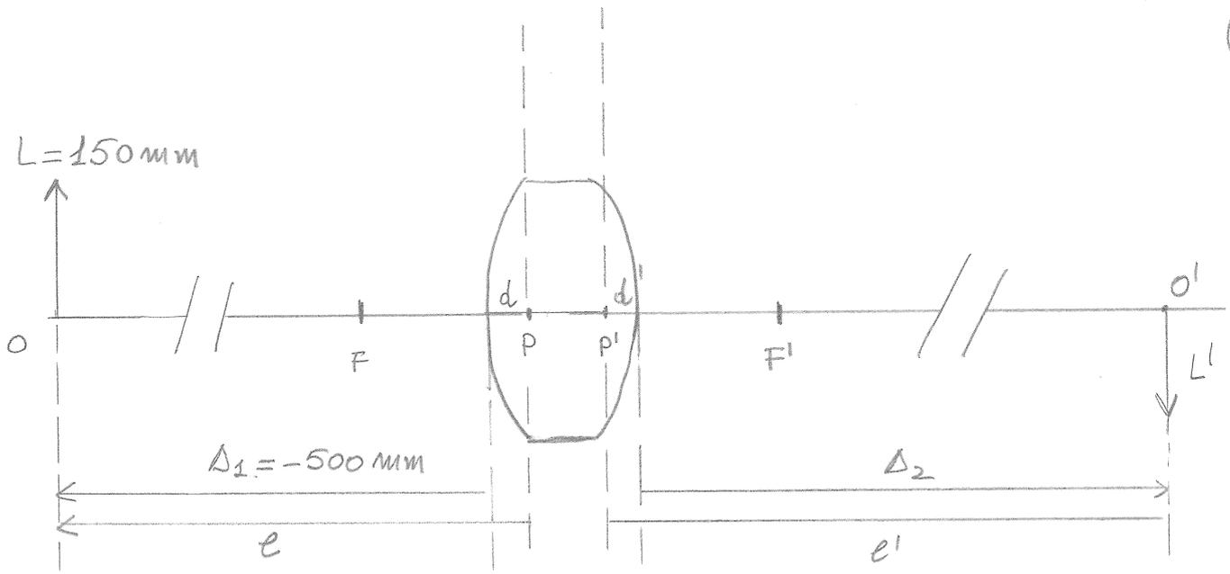
$$l = \Delta_2 - d \quad ; \quad \frac{1}{e'} = \frac{1}{e} + \frac{1}{f'} \quad ; \quad \frac{1}{e'} = \frac{1}{\Delta_1 - d} + \phi \Rightarrow e' = 436.58 \text{ mm}$$
