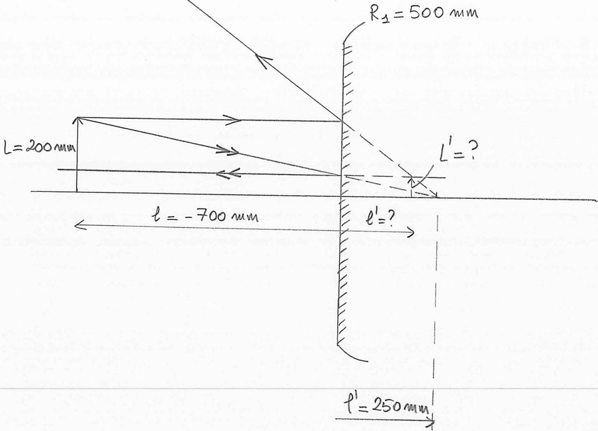
$$\frac{1}{e'} = -\frac{1}{e} + \frac{1}{f'} \Rightarrow \frac{1}{e'} = \left( \frac{1}{700} + \frac{1}{250} \right) \frac{1}{\text{mm}} \Rightarrow \boxed{e' = 184.21 \text{ mm}}$$
